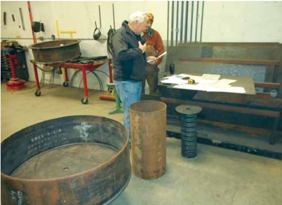
Building the bench-scale pilot furnace for testing magnesium ore. Photo courtesy Nevada Clean Magnesium Inc.
